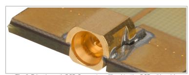
Fig. 1: Edge Launch PCB Connector affixed to the PCB with solder
